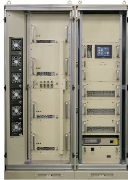
1428MHz High Stability Solid State Power Amplifier
